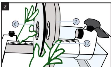
Remove the movable cutting element (6) of the knife block from the cutting unit (7) by pulling it slightly in the area of the recessed grips (17).
