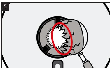
Check the knives for damages. If necessary, defective knives should be replaced.
