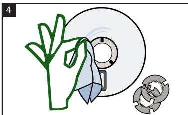
Clean the contact surfaces of the cutting unit and the blades with a clean, lint-free cloth.
