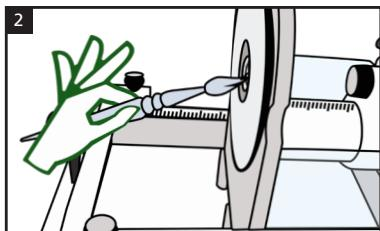
Now clean the machine using a commercially available brush. Pay special attention to the spaces between the blades and all other moving parts. Make sure to clean both cutting elements thoroughly.
