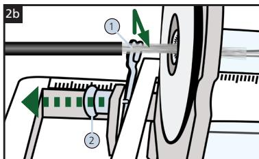
The cable support (1) is held in the working position by a locking bolt (2). By pulling the locking bolt, the cable support can be swivelled to the side when not in use.
