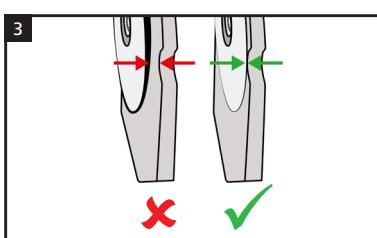
The cutting elements should be mounted with as few gaps as possible between them. mounted to each other.
