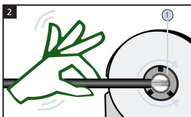
To cut the shield, guide the stripped cable through the cutting elements (7) up to the stop (10). By moving the cable with slight pressure (clockwise and anticlockwise) along the inside blades, the braided shield is cut.
