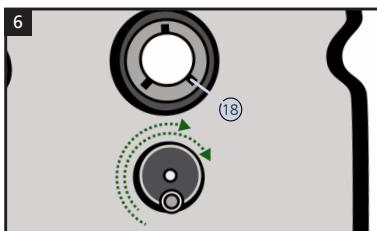
Turn the inner ring of the ball bearing (18) several times, to build up an even lubricating film.
