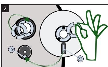
The backs of the knives should be moistened with precision mechanic's oil. Now join the two cutting elements together. Make sure that there are no foreign bodies between the surfaces (**ATTENTION:** danger of crushing). The eccentric guide (23) of the running disc must be positioned over the cam (19) of the eccentric bearing. It is recommended to set the centring cam to approx. 6 o'clock.
