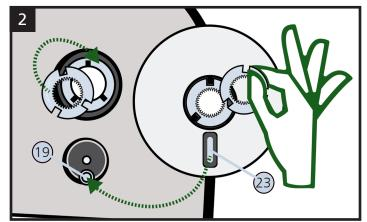
The backs of the knives should be moistened with precision mechanic's oil. Now join the two cutting elements together. Make sure that there are no foreign bodies between the surfaces (ATTENTION: danger of crushing). The eccentric guide (23) of the running disc must be positioned over the cam (19) of the eccentric bearing. It is recommended to set the centring cam to approx. 6 o'clock.
