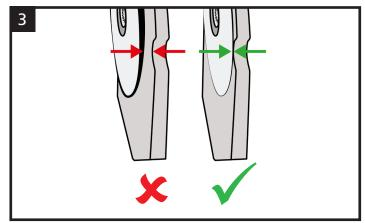
The cutting elements should be mounted with as few gaps as possible between them. mounted to each other.
