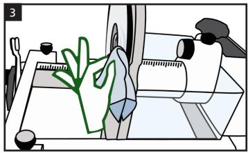
If necessary, the machine can also be cleaned with a damp cloth. Push the movable stops on the guide backwards and tilt the complete unit forwards to transport the shield braids to one side of the collection tray. Remove the braid residues from the collection tray using a hoover.
