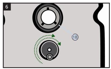
Turn the inner ring of the ball bearing (18) several times, to build up an even lubricating film.
