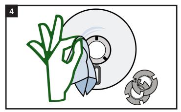
Clean the contact surfaces of the cutting unit and the blades with a clean, lint-free clothblades with a clean, lint-free cloth.
