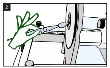
Now clean the machine using a commercially available brush. Pay special attention to the spaces between the blades and all other moving parts. Make sure to clean both cutting elements thoroughly.
