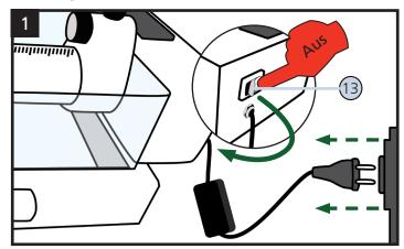
Switch the machine off using the on/off switch (8) and disconnect it from the mains.
