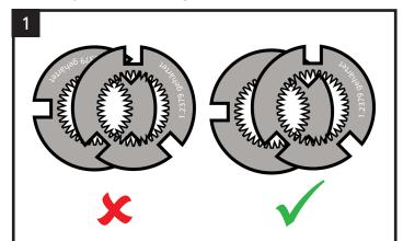
Position one knife each in the recess of the two cutting elements. The three grooves of the knives (21) engage in the respective driver bars (20). The flat (unlabelled) backs of the knives face each other.
