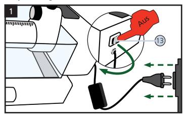
After using the machine, it must be switched off (13) and disconnect it from the mains supply.
