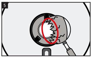
Check the knives for damages. If necessary, defective knives should be replaced. Spare part no. 8078856.
