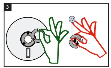
Remove the knives (22) from the cutting elements (CAUTION: danger of cutting).
