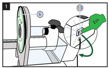
The motor is switched on via the on/off switch (13). The movable cutting element (6) starts to oscillate/vibrate.
