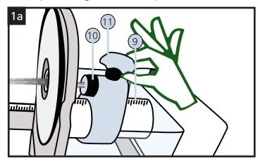
The length of the braided screen to be cut off is determined by the the length stop (10). The corresponding dimension is set on the scale (9). For adjustment use the back of the length stop, which is fixed with the fixing screw (11). The maximum length can be 50mm.
