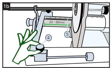
The scaling **(5)** on the front linear guide defines the length of the remaining braided shield (range 20 to 90mm). The length is set between the end of the jacket and the end of the braided shield. For adjustment, the back of the length stop is used, which is to be fixed by means of the two knurled screws **(4)**.
